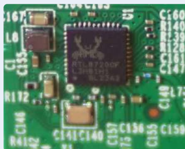
Figure 31. MCU RTL8720CF de Realtek.
